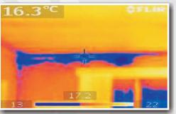
Moisture intrusion in the attic. Here it saturated the top of this inside wall. Eventually it will affect the entire wall and the picture window frame.
