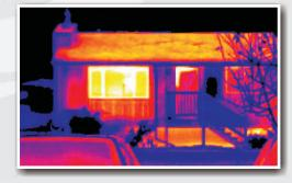
This winter thermogram shows inadequate roof insulation, an uninsulated basement, a door seal leak and poor wall insulation behind a baseboard heater under the window.
