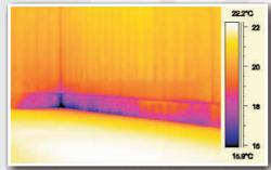
The carpet was replaced because of a water leak but they neglected to scan the wall for the "wicking" effect which left the wall moist and produced an ideal environment for mold, mildew and pests.
